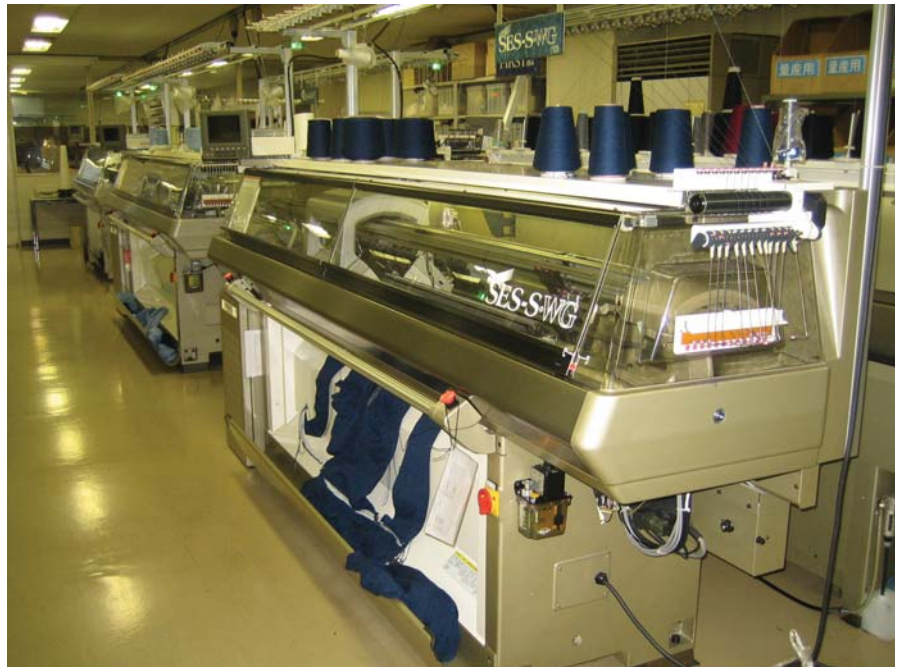
Shima's fully automatic, seamless flat-knitting machines called wholegarment knitting machines
